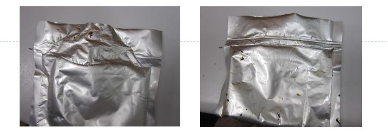
Two pictures show two sides of the same pouch. The sealing was damaged on one side compared to the one on the right.
