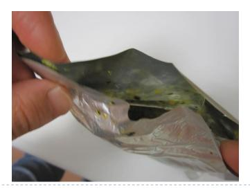
This is the same pouch as shown above. The plastic layers were separated. There is a hole in the picture. Two layers around the hole were originally adhered together as one side of retort pouch.
